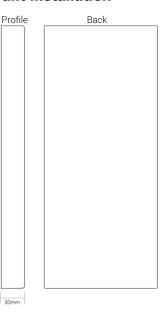
**Chassis:** Aircraft Grade Anodized Aluminum with Curved Sleek Profile **Dimensions:**  $314 \times 140 \times 30 \text{mm}$
